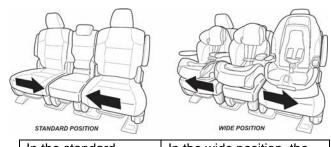
In the standard In the wide position, the position, the seats seats are located outward are located inward for: for: Installation of Easier three car seats in • access to the the second row. third row. Additional hip Maximizing and shoulder second row room for outer seat passengers in the second row passenger headroom. seats.
