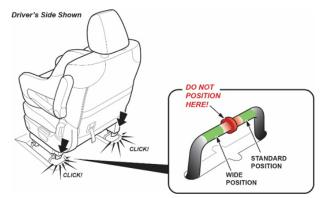
If despite the risks you choose to tip the entire second row seat forward to access the third row, make sure the seat is in the standard or wide position when lowering and latching the seat.
