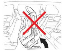
Honda does not recommend using this method to access the third row seats. When the second row outer seat is tipped forward, the seat may slide into the area between the standard and wide positions that prevents the seats from latching. Therefore, using this method of access increases the risk of having an unsecured second row outer seat.
