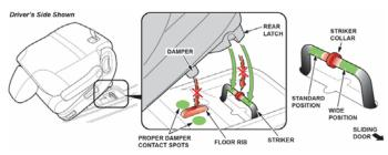
4. Press down on the rear part of the seat to set both rear latches. The latches click as they engage the floor strikers.
